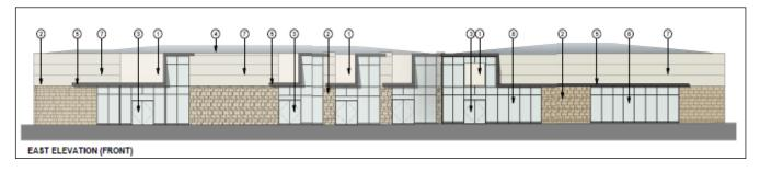
The schedule of materials for these units includes horizontal metal cladding above a stone effect cladding at lower levels for the walls of the buildings, powder coated frames for doors and windows and a composite roof panel arrangement.
